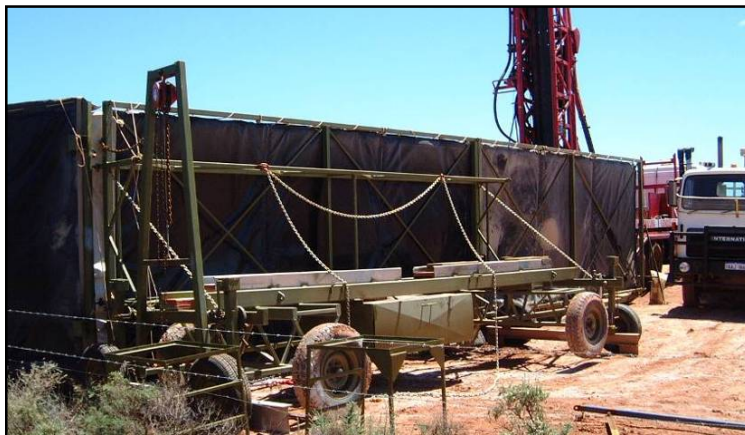
Figure 5 Drill Rig Acoustic Screen
